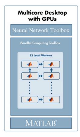
Note that, during training, the calculation of network outputs, performance, gradient, and Jacobian calculations are parallelized, while the main training code remains on one worker.
