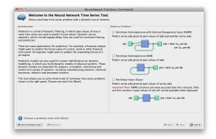
Network diagrams shown in the Neural Time Series Tool, Neural Training Tool, and with the view(net) command, have been improved to show tap delay lines in front of weights, the sizes of inputs, layers and outputs, and the time relationship of inputs and outputs. Open loop feedback outputs and inputs are indicated with matching tab and indents in their respective blocks.
